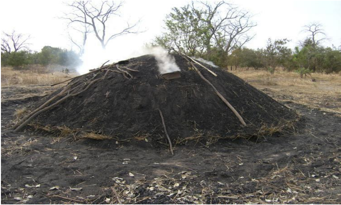
Figure 2.XX: Earth mound method of charcoal production being used in Mau West Forest
