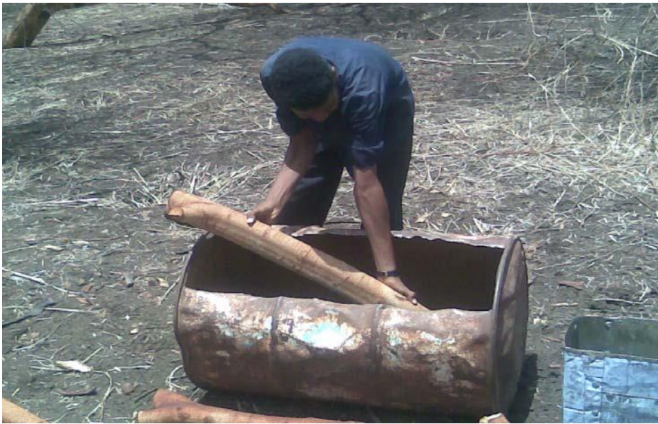
Figure 2.XX: Oil drum kiln
