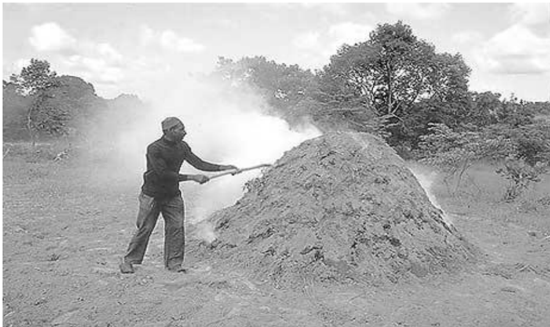
Figure 2.X: Earth mound method of charcoal production being used in the Mau West Forest
