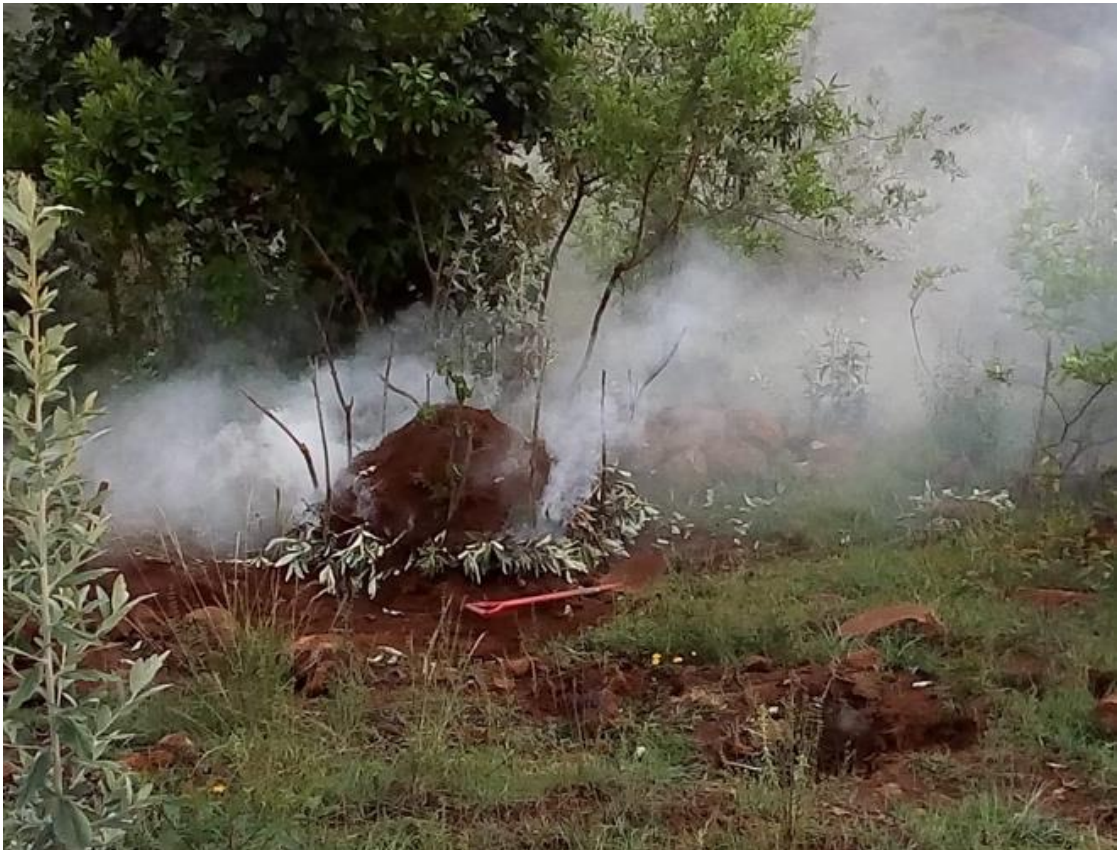
Figure 1.2: Traditional earth mound kiln in one of the study areas.
